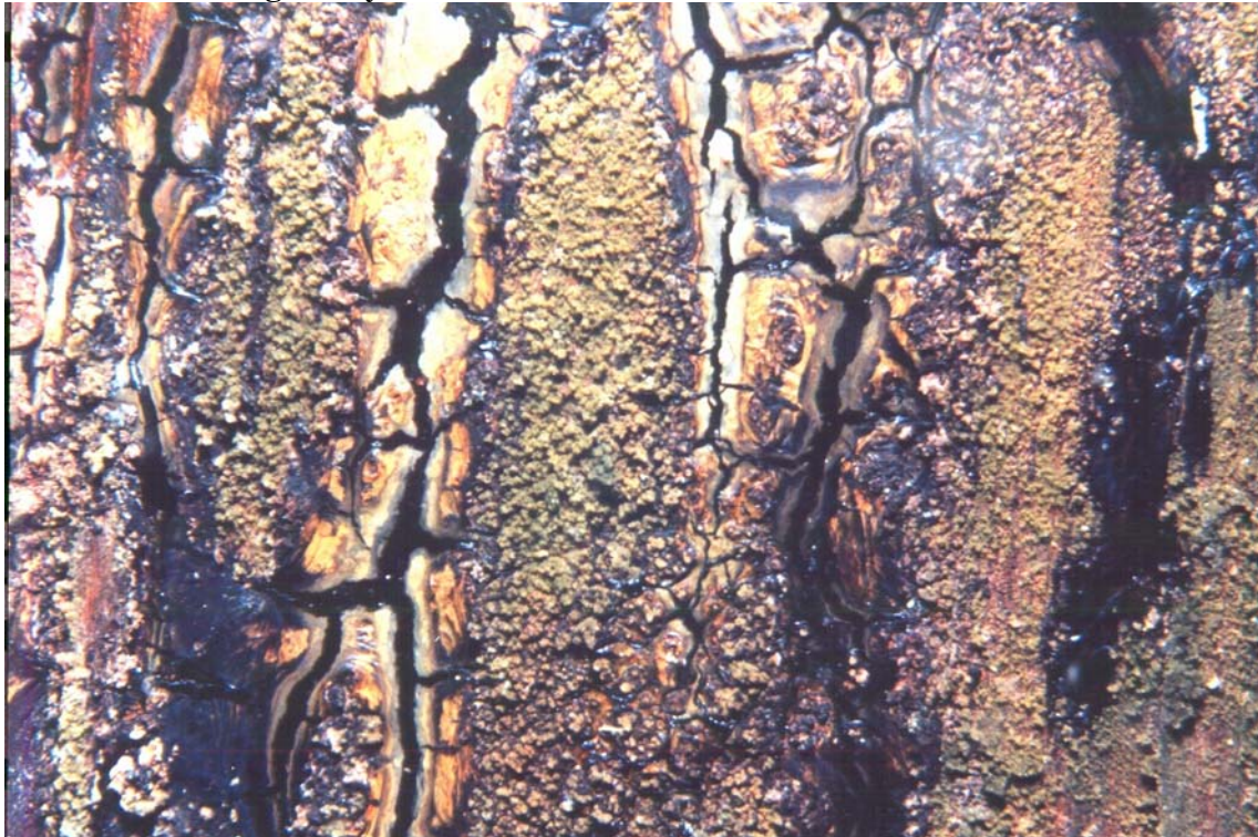
Plate 4. Magnified view of the BMP piling surface taken at +8' Chart Datum four years after construction – October 1999
