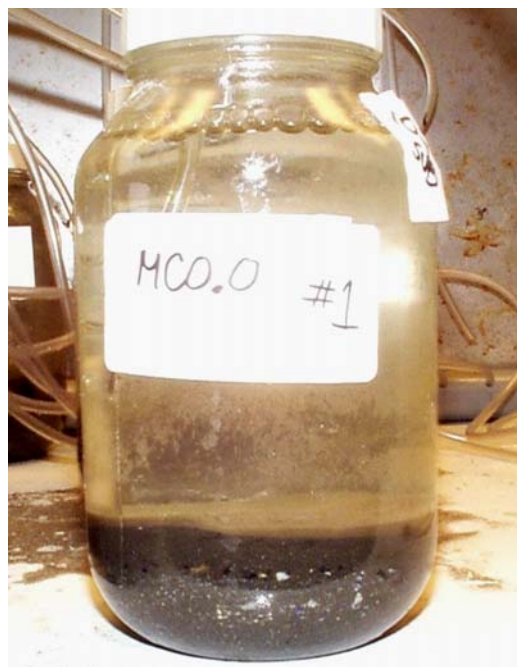
Figure 14. Bioassay Test Jar Taken at the End of the Pre-aeration and Bioassay Period. Note the layer of fine oxidized sediment on the surface
